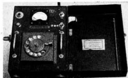
Fig. 6. Radio control transmitter constructed and used by the author. Note telephone dial for pre-selector keying. Circuit is similar to that in Fig. 5.
